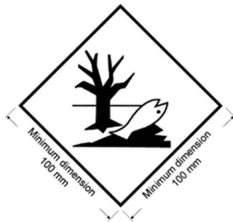
Environmentally hazardous substance mark
